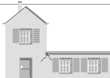
Crack control in irregular elevations (Page 22)
