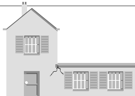
Crack control in irregular elevations (Page 22)
